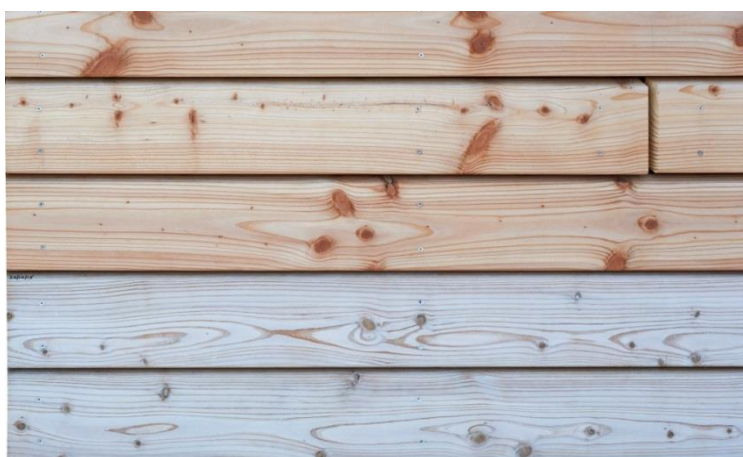
RW014 open rainscreen Scotlarch® after ten months weathering NE aspect. Above: No SiOO:X applied. Below: SiOO:X applied.
